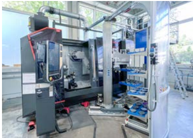
With workpiece pool for unmanned production
