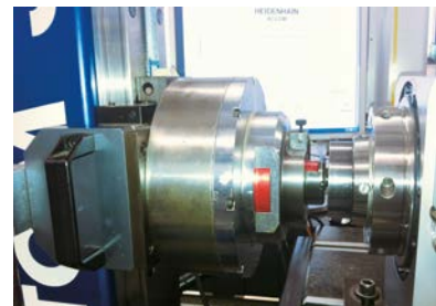
Measuring the indexing accuracy – fully automatically
